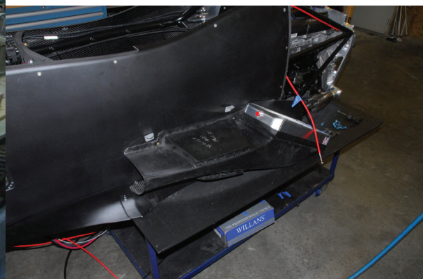
BELOW The carbon radiator ducts also act as a side impact structure with carbon beams bonded top and bottom
