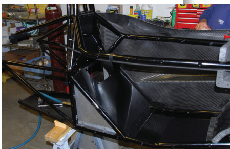
BELOW The tubeframe is still central to the chassis function. Here the cockpit ‘inner’ panels are fitted to the far side. Note that the frame runs right through the engine bay
