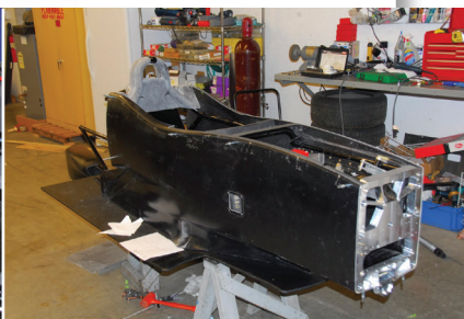
BELOW Once clothed with inner and outer cockpit panels, the tubeframe is effectively hidden
